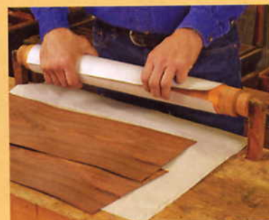
Cut the veneer to size. Make a paper template rather than bending the dry, brittle veneer. The veneer should overlap \frac{1}{2} in. at the seam.
