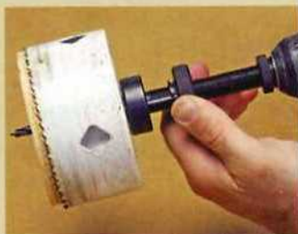
Ease out the plug. To remove a plug from a hole saw using the Twister ezeOUT, simply squeeze the drill's trigger.
