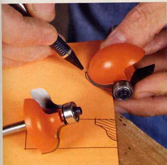
Make templates. Trace the profile of each router bit on thin cardboard to create templates for the molding.
