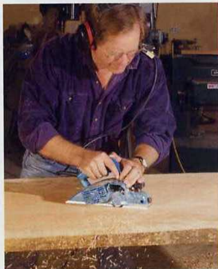
Watch chip output to determine flatness. Set the planer to a lighter cut. If the surface is flat, the planer should send out a steady stream of fine shavings.
