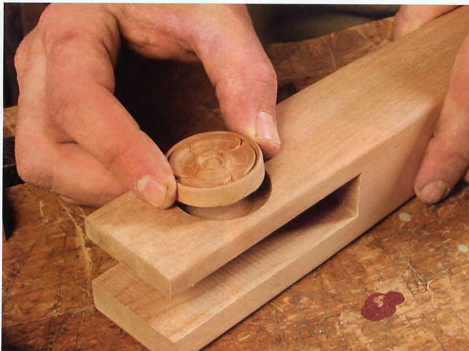
Highlighting a leg. By inserting the rosette into a perfectly matched hole, it appears that the leg itself was carved.
