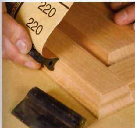
Rubber profiles. Using a rubber pad that fits the molding helps keep the edges of the profile sharp.
