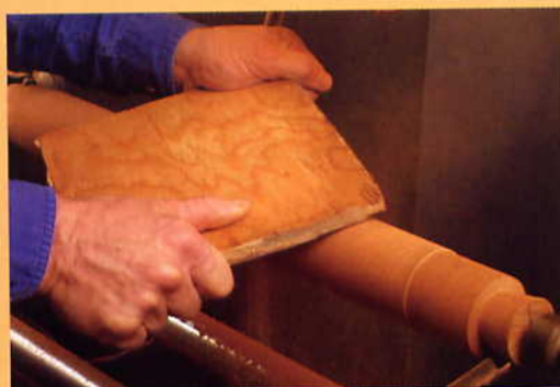
Turn a straight column and secure it well. Glue cloth-backed sandpaper to a square of plywood to make a low-tech smoother for turnings. To secure the column, make a set of extralong benchdogs (right), with a screw tip poking out of each. Also, tape off the tenon areas of the column.
