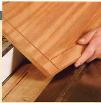
Establish the field. Score a 3/16-in.-deep shoulder around the field using the tablesaw.
