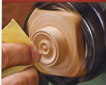
Rosette blanks turned on a lathe have a limitless number of profile and size possibilities.
